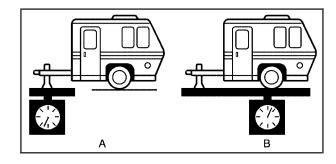
The trailer tongue weight (A) should be 10 percent to 15 percent of the total loaded trailer weight, up to a maximum of 500 lbs (226 kg) with a weight carrying hitch.
